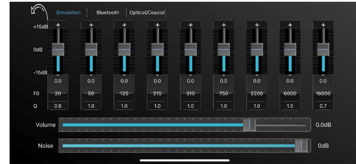
Depending on the source it might be necessary to flatten the input signal to receive an accurate sound signal. This could be necessary especially in cars with basic OE speaker system without separate tweeters. Some of the OE headunits of those cars are provided with an extreme treble volume to get more treble sound out of the broadband speaker.
