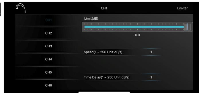
The limiter function is the reinsurance if you drive your car stereo hard on the limit. Turn up the volume until you listen to distortion of the sound, especially the woofers and subwoofers. Now choose the limit (db) value how much the limiter should reduce the sound volume level, choose the speed how quickly the limiter shall reduce the sound volume level and finally how long the limiter shall reduce the sound volume level.
