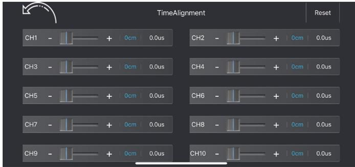
In this menu you can apply a time delay to the speaker signal to simulate an ideal listening position.
