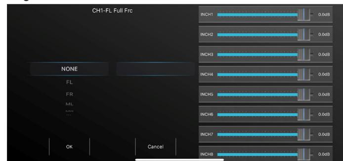
In this menu you can assign an input signal to each output channel – including desired gain level. It is also possible to combine two or more input signals to one output channel. For better convenience you can additionally label each channel.
